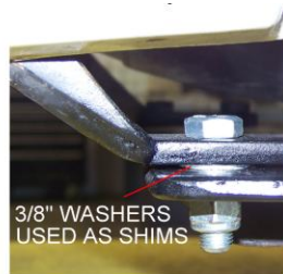
ILLUSTRATION OF SHIM PLACEMENT BRACKET PICTURED MAY NOT MATCH YOUR BRACKET
