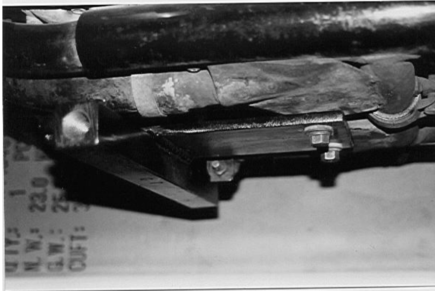
KAWASAKI KZ 1100 BELLY BRACKET INSTALLED (LEFT SIDE)
