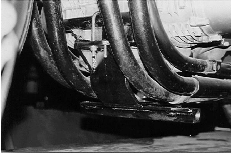
KAWASAKI KZ 1100 BELLY BRACKET INSTALLED (FRONT VIEW)
